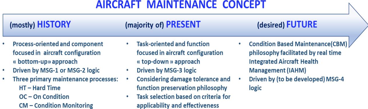
Figure 3: Driving Factors in Scheduling Maintenance
